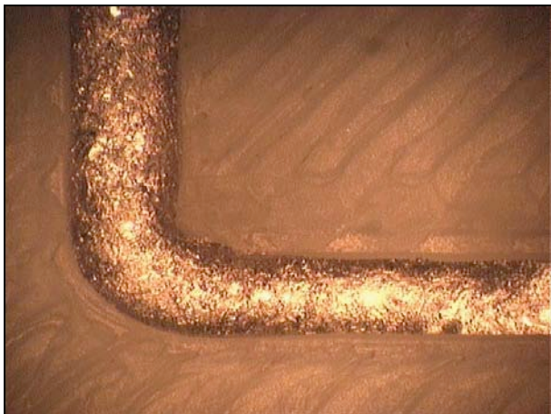
Figure 10: Magnification of forged circuit around 90 ° bend (channel width 1.2 mm). Circuit is consistent throughout and does not suffer from overspill
