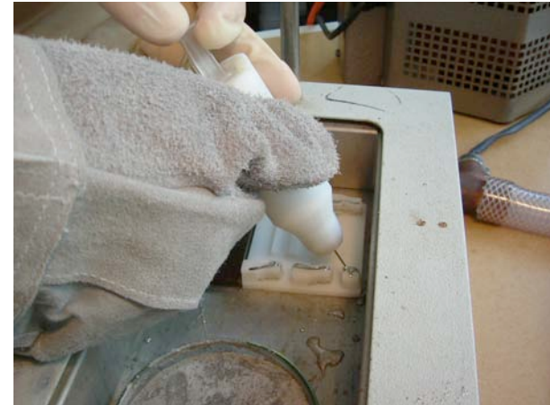
Figure 9: Injection process into component on hotplate. Note molten alloy supply in petri dish also on hotplate.
