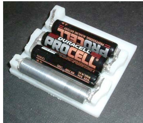
Figure 13: Battery case. Push fit on batteries maintained by battery terminals on spring clips.
