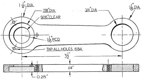
Fig. 18. The connecting-rod
