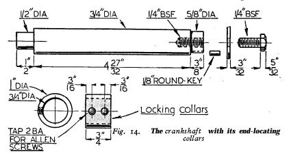
in need of reaming, for it may be taken into consideration that the crankshaft runs at only some 90 r.p.m. and the large bearing surfaces provided are only lightly loaded. As a matter of interest, the bearings were actually bored with a  $\frac{1}{16}$  in. diameter boring bar furnished with a single inset cutter, and the tool marks were removed from the bearing surfaces by taking a series of very fine cuts with an adjustable hand reamer.
