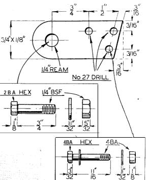
Above-Fig. 21. The small-end bearing bracket with its bolt fittings
