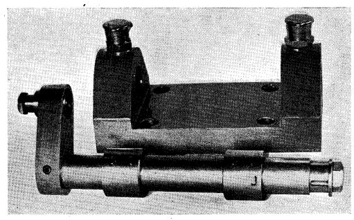
Fig. 15. The complete crankshaft assembly with its bearing bracket
