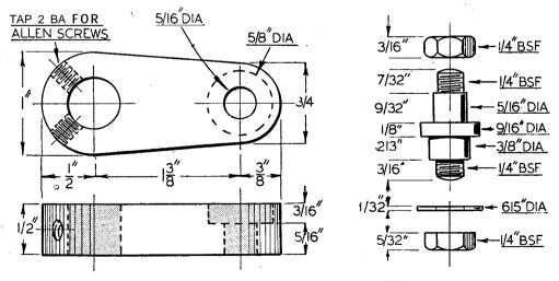
Fig. 17. The crank web and its crankpin
