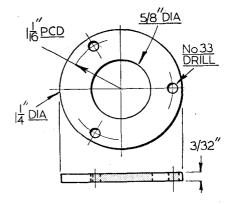
Fig. 19. Pressure plate for securing the big-end ball-race
