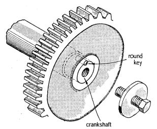
Fig. 16. Method of securing the gear wheel to the crankshaft
