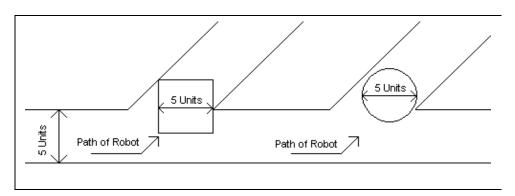
*Fig. 1.1 A circular base can fit into smaller passages than a square base without precise reorientation*
