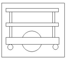
Fig 1.2 A layered mounting system provides a way to easily add and remove subsystems independently.
