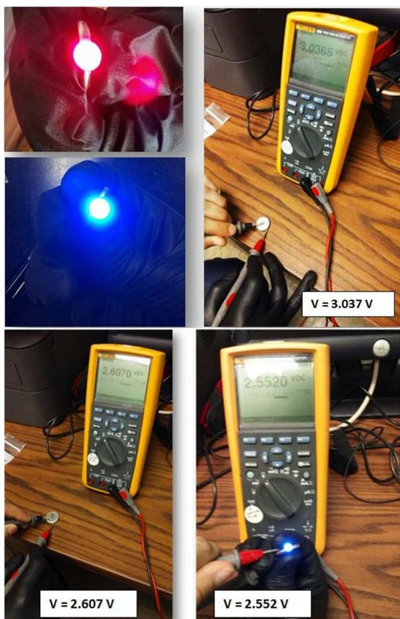
Fig. 9 (a) A red and a blue LED lit by a Li-MnO<sub>2</sub> coin cell at  $V > 3.0$  V and (b)  $V_{OC}$  of a Li-S coin cell without and with production of blue LED light.
