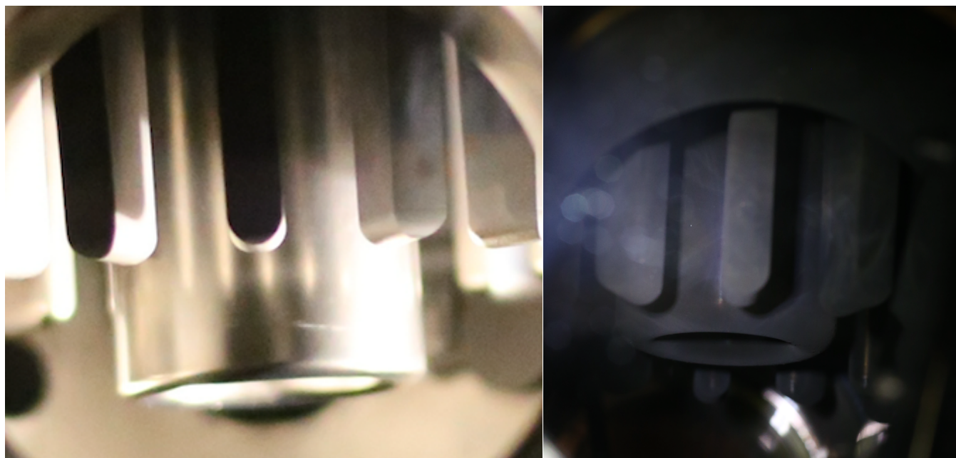
Figure 2. Our 2021 polished anode (left) still shined mirror-bright after three shots in August, 2021. It is viewed through a window on our vacuum chamber. The anode is a bit more than two inches in diameter. The colors on the anode seen here are the result of lighting and camera response. The true color of the anode is still silver. In contrast, our first beryllium anode after one shot in 2019 (right) was covered with a dark "snow" of beryllium oxide dust, which was vaporized and redeposited by FF-2B's powerful electric currents. This is what we avoided by our new polishing procedure.
