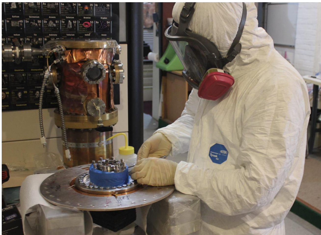
Dr. Syed Hassan, in full protective gear, does final preparation to put the new beryllium anode plate (with anode hidden underneath) onto the FF-2B device.
