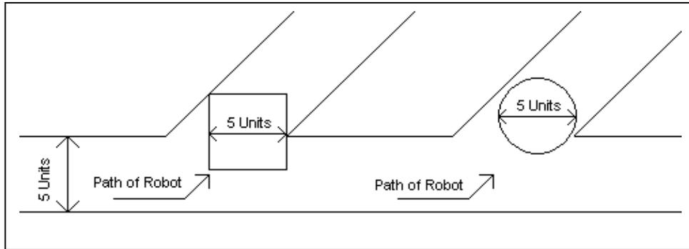
*Fig. 1.1 A circular base can fit into smaller passages than a square base without precise reorientation*
